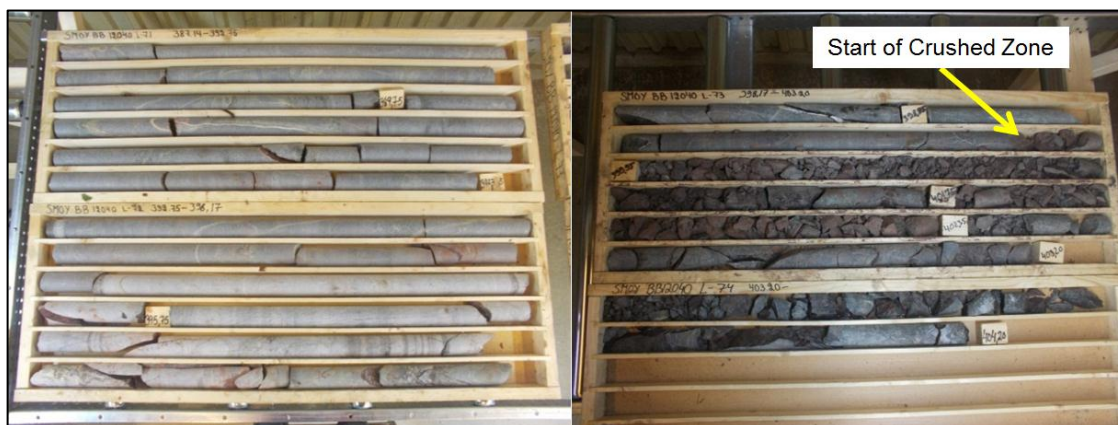
Figure 10-3: Core Log from BB12003 showing typical Core (left) Entering Crush Zone (right) (Source: SRK, 2014)
