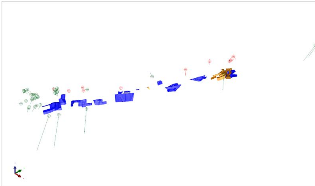
Figure 4, The relogged drillholes at Håksberg in relation to the reconstructed ore wireframes.
